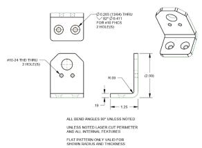
0.015" chamfer or radius is required on all sheet metal edges.
